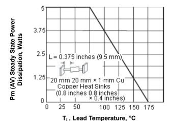
Fig. 5-Steady State Power Derating Curve
