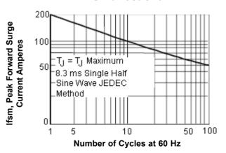
Fig. 6-Maximum Non-Repetitive Peak Forward Surge Current Unidirectional
