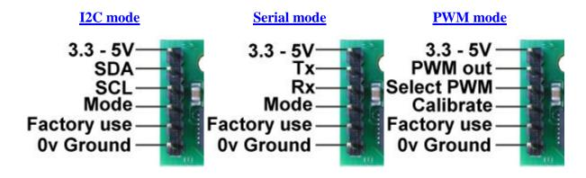
To enter the I2C mode of operation leave the mode pin unconnected
