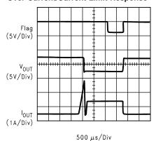
\* Output is shorted to Ground through a 100  $\text{m}\Omega$  resistor
