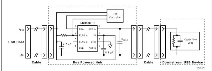
FIGURE 4. Soft-Start Application (Single port shown)
