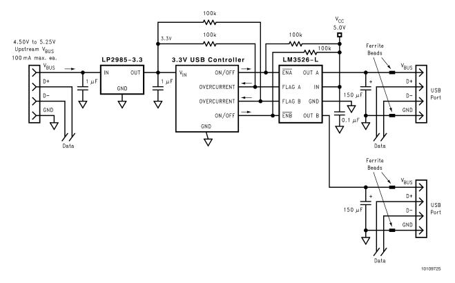
FIGURE 3. Dual-Port USB Self-Powered Hub
