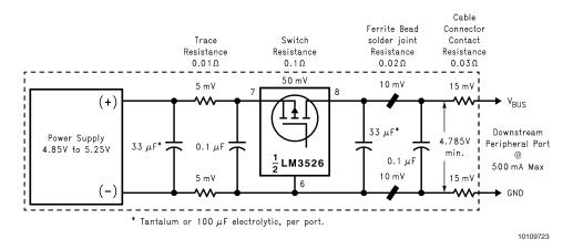
FIGURE 2. Self-Powered Hub Per-Port Voltage Drop
