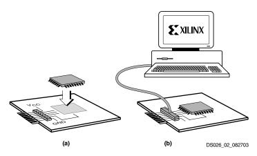
Figure 3: JTAG In-System Programming Operation
