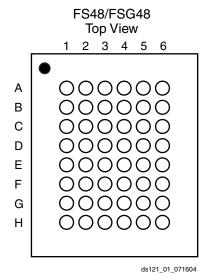
Figure 17: FS48/FSG48 Pinout Diagram (Top View)
