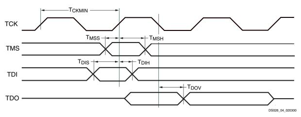
Figure 4: Test Access Port Timing
