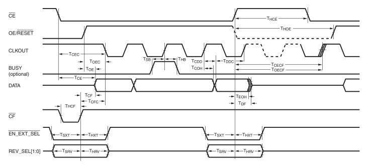
$\label{eq:Note: 8 CLKOUT cycles are output after $\overline{\text{CE}}$ rising edge, before CLKOUT tristates, if OE/$\overline{\text{RESET}}$ remains high, and terminal count has not been reached.}$
