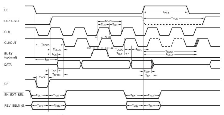
$\label{eq:Note: 8 CLKOUT cycles} \textbf{Note: 8 CLKOUT cycles} \ \text{are output after } \overline{\text{CE}} \ \text{rising edge, before CLKOUT tristates, if OE/RESET remains high, and terminal count has not been reached.}$
