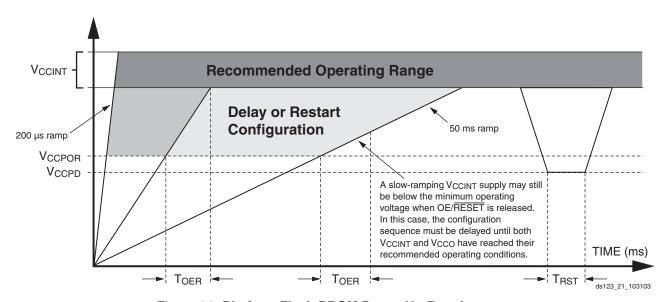
Figure 14: Platform Flash PROM Power-Up Requirements
