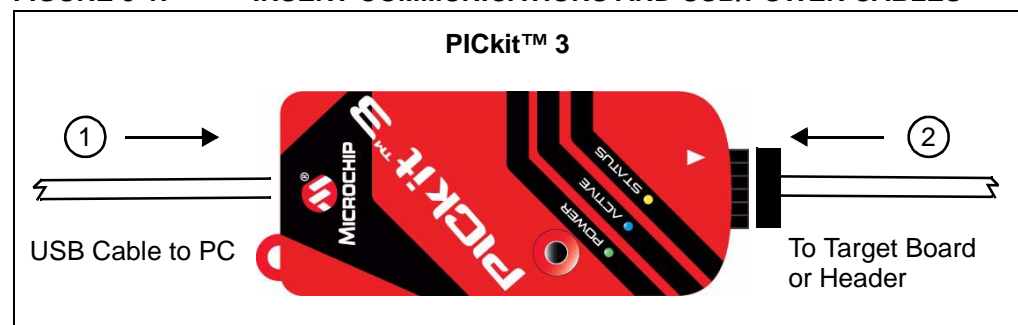
FIGURE 3-1: INSERT COMMUNICATIONS AND USB/POWER CABLES
