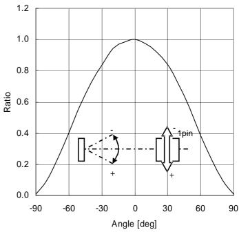
Figure 4. Directional Characteristics 2
