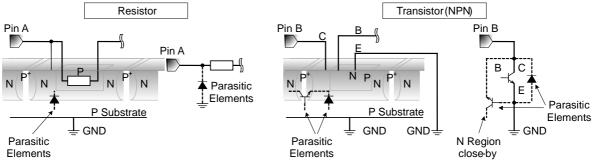
Figure xx. Example of monolithic IC structure
