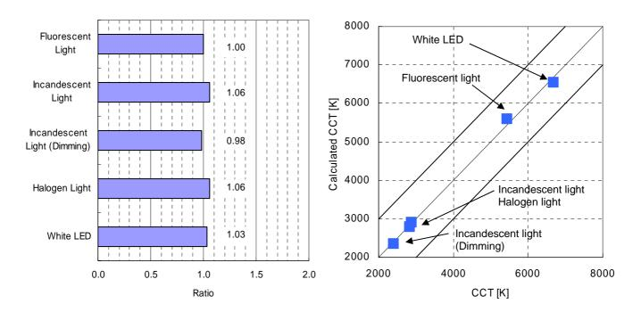
Figure 5. Light Source Dependency of lx calculation from RGBC (Fluorescent Light is set to "1")
