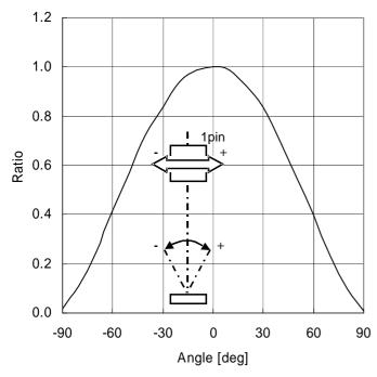
Figure 3. Directional Characteristics 1
