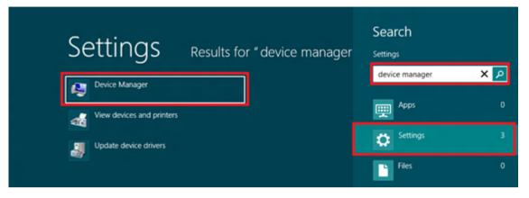
Plug-in the USB device (PL2303HXA/XA) to the USB port. If the PC is connected to the Internet, Windows will first check Windows Update for new driver available. It will download the new driver instead which is not compatible with PL2303HXA/XA and will show a yellow mark (error code 10) for "Prolific USB-to-Serial Comm Port" in Device Manager.
