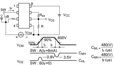
$C_{ML}$  ( $C_{MH}$ ) is the maximum rate of rise (fall) of the common mode voltage that can be sustained with the output voltage in the low (high) state.
