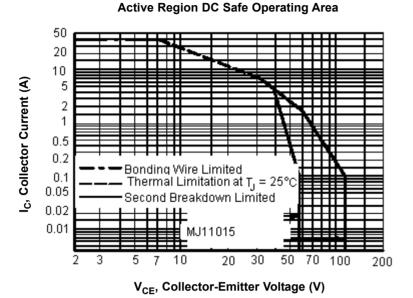
There are two limitations on the power handling ability of a transistor average junction temperature and secondary breakdown. Safe operating area curves indicate  $I_C - V_{CE}$  limits of the transistor that must be observed for reliable operations e.g., the transistor must not be subjected to greater dissipation than the curves indicate.
